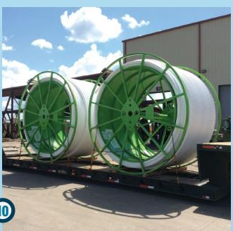
The project was completed on October 23, 2015. As the wellhead was over 8,600' from the tank battery, the flowline and power fluid lines were run together. The total pipeline length was 17,230' of 2 1/2" nominal ID (2 7/8" actual OD) Schedule 40 0.203" WT A53/X52C/X65C grade coiled line pipe. The pipe was delivered on six uninterrupted reel lengths of up to 3,100' each. (Pic 10)
