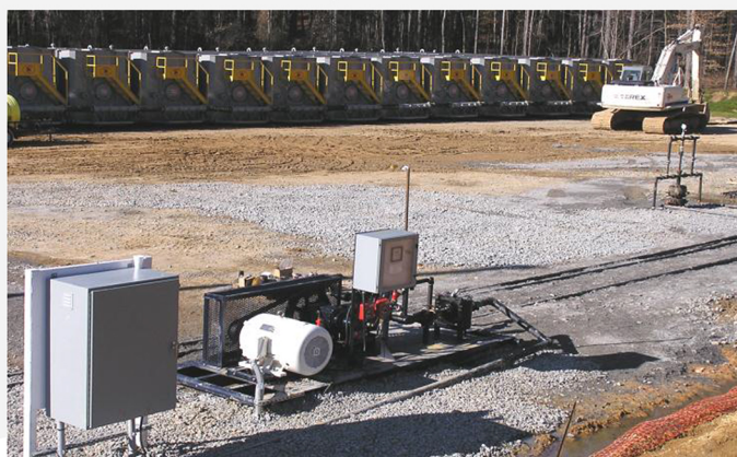
Shown Above: JJ Tech utilizes a diaphragm pump which has no seals or packing unlike a traditional triplex plunger pump. The seal-less design reduces downtime and maintenance while keeping the location free of lubricating oil and salt water. The T8045 diaphragm pump is capable of 3000 psi at 1550 bpd.
