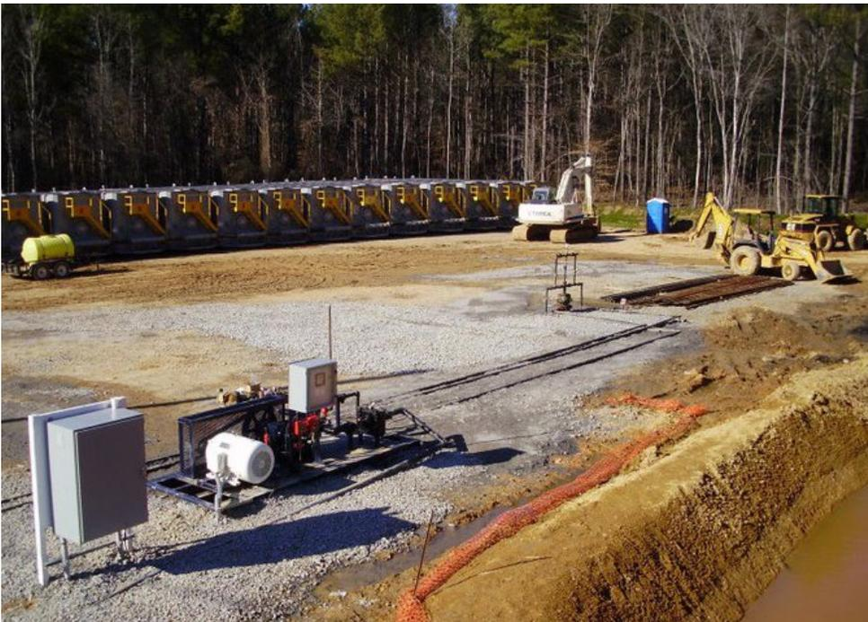
JJ Tech utilizes a diaphragm pump which has no seals or packing unlike a traditional triplex plunger pump. The seal-less design reduces downtime and maintenance while keeping the location free of lubricating oil and salt water. The T8045 diaphragm pump is capable of 3000 psi at 1550 bpd.
