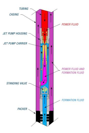
The jet pump is set in the tubing string above a packer which is set just above the perfs. Power fluid (water) is injected down the tubing through a nozzle. Power fluid and produced fluid are combined in the throat (Venturi Effect) and return up the annulus.
