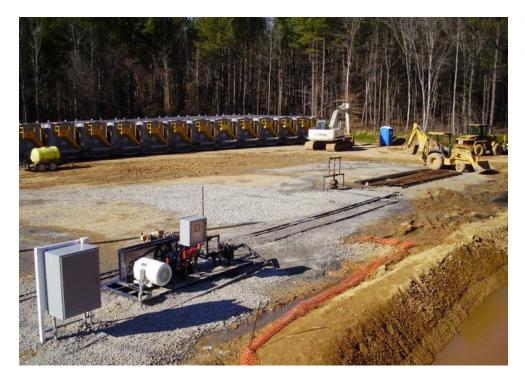
JJ Tech utilizes a diaphragm pump which has no seals or packing unlike a traditional triplex plunger pump. The seal-less design reduces downtime and maintenance while keeping the location free of lubricating oil and salt water. The T8045 diaphragm pump is capable of 3000 psi at 1550 bpd.
