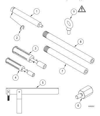
WARNING: Item 9, M10 Diaphragm Plate Eyebolt is used to lift Diaphragm Plate (52) only. Do not use to lift entire pump. Attempting to lift entire pump with Eyebolt (9) may cause personal injury or damage to equipment.
