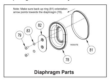
a. See Diaphragm Parts View. Remove two screws (79), two O-rings (83) and follower (82).
